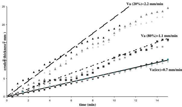
Figure 4. Measurements of eroded thickness of pure ice and sandy permafrost with different ice contents, initially at  $-7.5^{\circ}\text{C}$ , heated by a turbulent water flow (5.5°C and  $Re=15\ 900$ ). In 10 minutes, the measured eroded thickness are about 6 mm, 11 mm, 18 mm for pure ice, permafrost with  $\omega=80\%$  and  $\omega=20\%$  respectively. Linear fit gives measured erosion rates equal to 0.7 mm/min, 1.1 mm/min
