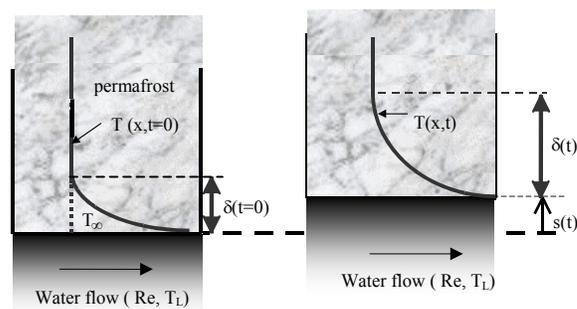
Figure 1. (a) The initially isothermal permafrost ( $T_{\infty}$ ) is suddenly heated by a permanent water flow ( $Re, T_L$ ). After a rapid transient phase, the interface reaches the melting temperature ( $T_m=0^{\circ}C$ ). Then, the thermal erosion initiates and the interface starts to move. (b) The interface progressively moves. Its instantaneous position and erosion rate are given by  $s(t)$  and  $ds/dt$ . The instantaneous thickness of the thermal boundary layer is  $\delta(t)$ .
