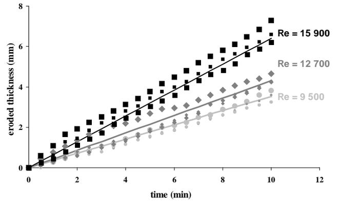
Figure 2. Measurements of eroded thickness of pure ice initially at  $-7.5^\circ\text{C}$ , heated by a turbulent water flow at  $5.5^\circ\text{C}$ . In 10 minutes, the measured eroded thickness of the ice sample are 3.5 mm, 4.5 mm, 6.5 mm for  $\text{Re}=9\,500$ , 12 700 and 15 900 respectively.
