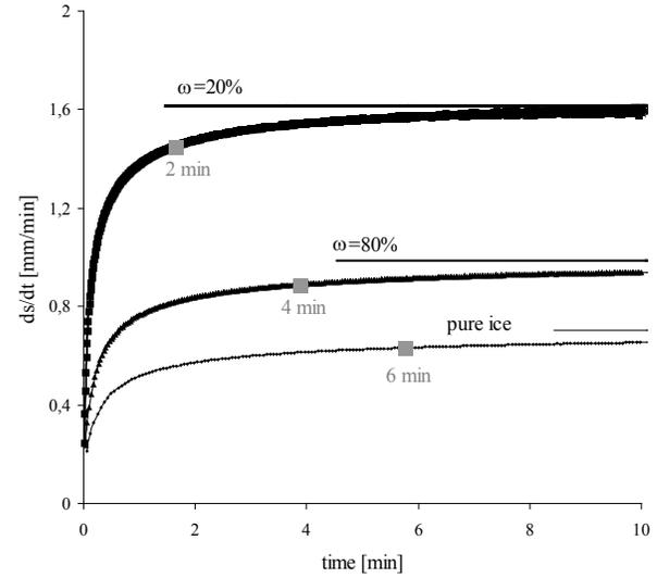
Figure 5. Theoretical erosion rate as a function of time for a water temperature equal to 5.5°C, an ice temperature equal to 7.5°C a Reynolds number equal to 15 900, applied to the geometry of our hydraulic channel. The erosion rate increases rapidly (acceleration phase) and stabilises (stationary phase). The smaller the ice content, the greater the erosion rate and the smaller the duration of the acceleration phase. Measured values are consistent with the asymptotic values.
