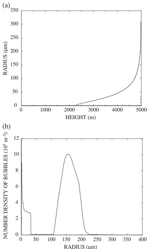
Fig. 11. (a) Evolution of bubble radius during ascent for the two population of bubbles (full stroke: first population and dashed stroke: second population). Note that the growth rate increases near fragmentation due to both effects of high decompression rate and high oversaturation. (b) Estimate of the size distribution at the fragmentation level. Note the fine population corresponding to tiny secondly nucleated bubbles. Parameters for this calculation are listed in Table 1.
