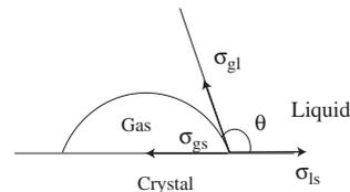
Fig. 2. Heterogeneous nucleation of a bubble on a plane liquid–solid interface (after Navon and Lyakhovsky, 1998). Coefficient  $\sigma_{gl}$ ,  $\sigma_{gs}$  and  $\sigma_{ls}$  are respectively the gas–melt, the gas–solid and the liquid–solid interfacial surface tension. Angle  $\theta$  is the wetting angle.
