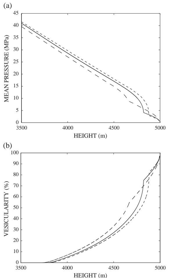
Fig. 7. (a) Evolution of mean pressure with height in the conduit for the three criteria (full stroke: gas volume fraction criterion, large dashed stroke: “Zhang criterion”, small dashed stroke: “Papale criterion”) and (b) Evolution of vesicularity with height. Note the differences in fragmentation height and vesicularity at fragmentation. Parameters for this calculation are listed in Table 1.
