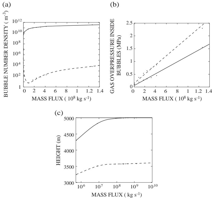
Fig. 5. (a) Bubble number density and (b) gas overpressure (full stroke: first population, dashed stroke: second population) as a function of mass flux of the eruption. (c) Fragmentation height (full stroke) and nucleation height (dashed stroke) as a function of mass flux of the eruption. Note that for all mass fluxes a second nucleation occurs. Parameters of these calculations are listed in Table 1.
