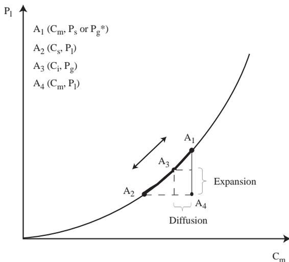
Fig. 1. (a) Schematic view of the processes of bubble growth. Below the solubility curve the dot represents one potential position of the magma during ascent on the  $(C_m, P_1)$  plot. When  $A_3(C_i, P_g)$  is near  $A_1$ , expansion is the dominant mechanism, when  $A_3(C_i, P_g)$  is near  $A_2$ , diffusion is the main mechanism.
