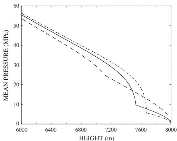
Fig. 13. Pressure profiles showing the evolution of the mean pressure for the three fragmentation criteria in the last 2000 m of the conduit (full stroke: gas volume fraction criterion, large dashed stroke: “Zhang criterion”, small dashed stroke: “Papale criterion”). Parameters used for calculation are in Table 2. Note that again, fragmentation occurs at a greater pressure in the case of “Zhang criterion”.
