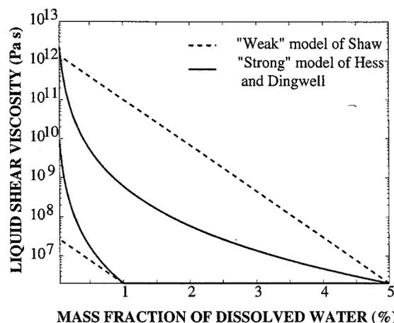
Fig. 5. Melt viscosity as a function of water content for a given starting viscosity. The two different viscosity functions have marked differences in the rate of viscosity variation with decreasing water content. At low initial volatile content, the ‘strong’ model predicts viscosities which are always higher than those of the ‘weak’ model. At large initial volatile content, the reverse is true.
