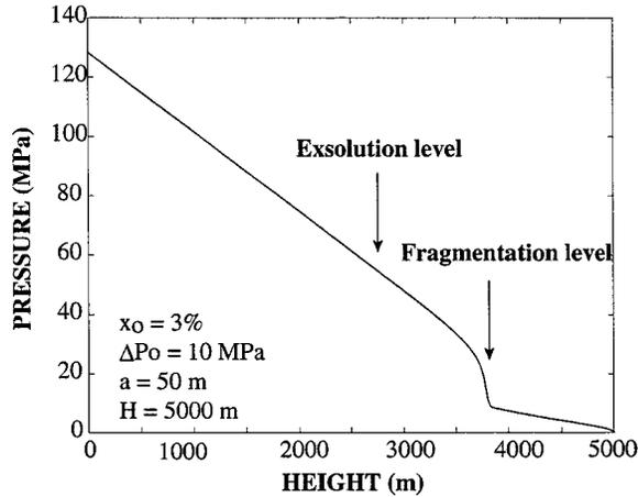
Fig. 3. Bulk flow pressure as a function of height in the conduit using the ‘strong’ viscosity function from [34]. Other parameters are listed in Table 1.
