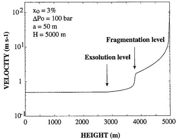
Fig. 4. Vertical velocity as a function of height in the conduit using the ‘strong’ viscosity function from [34]. Other parameters are listed in Table 1.
