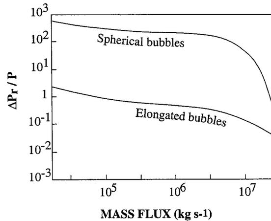
Fig. 10. The magnitude of horizontal pressure variations at the fragmentation level, scaled to the average flow pressure, as a function of eruption mass flux. In these calculations, the starting melt composition is the same and the starting melt viscosity depends strongly on water content as specified by [34]. The mass flux decreases with decreasing water content. Two different functions for the effect of bubbles on the bulk mixture viscosity are used. Parameter values are listed in Table 1.
