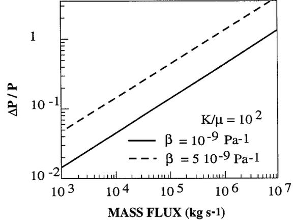
Fig. 11. Gas overpressure at the vent scaled to the pressure at the conduit wall as a function of eruption mass flux. The solution was with the simple analytical model valid for small compressibility. Parameter values are  $\mu = 10^7$  Pa s,  $\rho_0 = 2.4 \times 10^3$  kg m $^{-3}$ ,  $H = 1000$  m. The chamber pressure is  $P_0 = \rho_0 g H + \Delta P_0$ , with  $\Delta P_0 = 6.5$  MPa. The eruption mass flux varies as a function of conduit radius  $a$ .
