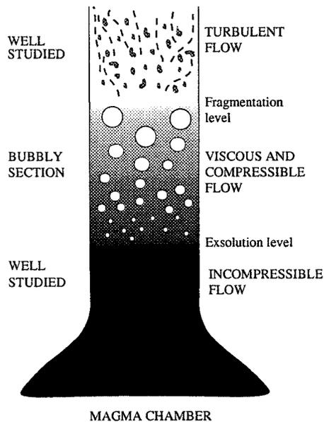
Fig. 1. Schematic representation of the different parts of the volcanic conduit. The intermediate region where bubbles nucleate and expand before fragmentation has not been investigated with the necessary degree of generality.
