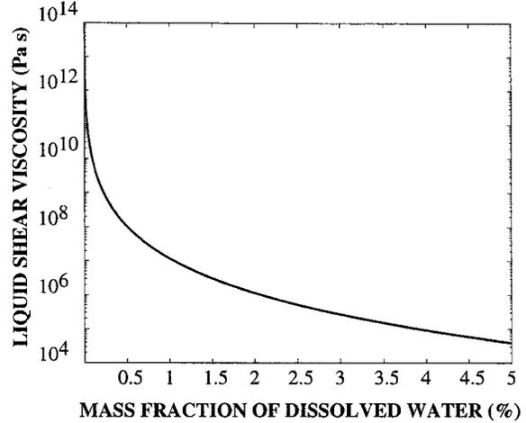
Fig. 2. Liquid viscosity as a function of water content for a leucogranitic melt. Data are taken from [34]. Note the very large viscosity variation when water contents are less than about 1%.
