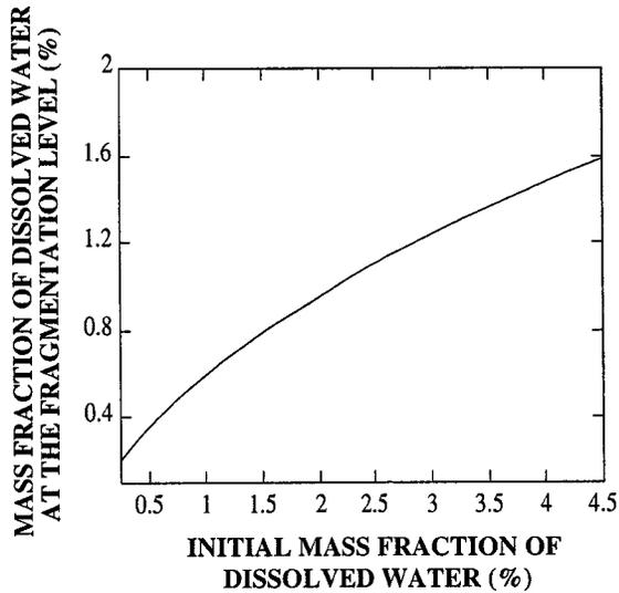
Fig. 6. Mass fraction of dissolved water at the fragmentation level. Parameters for the calculations are listed in Table 1.
